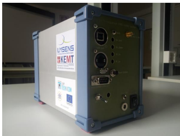
Fig. 6. Complete UWB sensor node with all components placed in aluminium box. Back panel contains SMA connector for RF antenna in SRD frequency band, power switch, diagnostic LEDs, configuration switches, USB and UART interfaces to be used for further firmware development.
