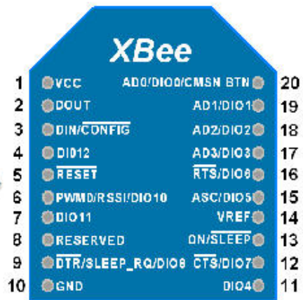
XBee Pin Configuration
